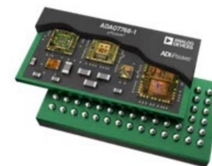
Figure 1: ADI's ADAQ7768-1  $\mu$ Module data acquisition system. (Image source: Analog Devices, Inc.)
