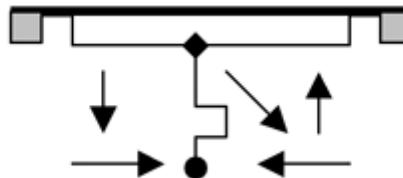
This type of activation is for picking up very small motions, and as a result, will generate very small outputs from the piezo bender, that must be greatly amplified.
