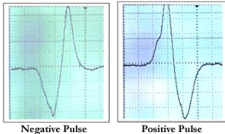
These signals were acquired using circumferential mounting and indirect pressures.
