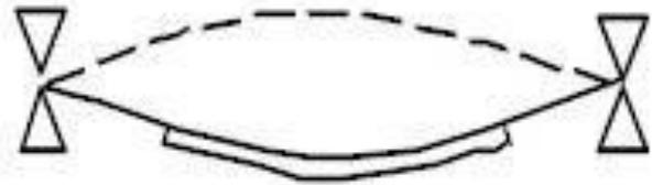
Mounting a piezo at the outer edge of its metal plate results in the widest usable bandwidth (overall frequency response). This mounting method distributes the impedance peak over a wider range and increases the moving surface area of the piezo, at the expense of peak SPL. Choose this mounting method when using a piezo to create tones at multiple frequencies.
