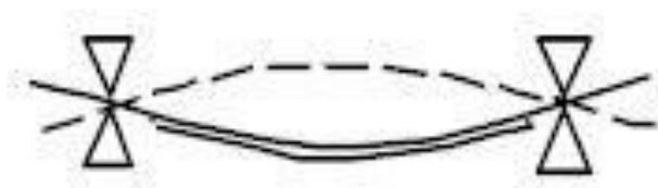
Mounting a piezo at its nodal point—just outside the diameter of the ceramic disc—results in the highest SPL at the expense of reduced bandwidth
