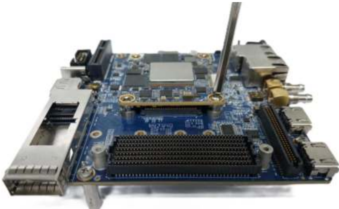
Figure 28: Removal SOM from Carrier Board
