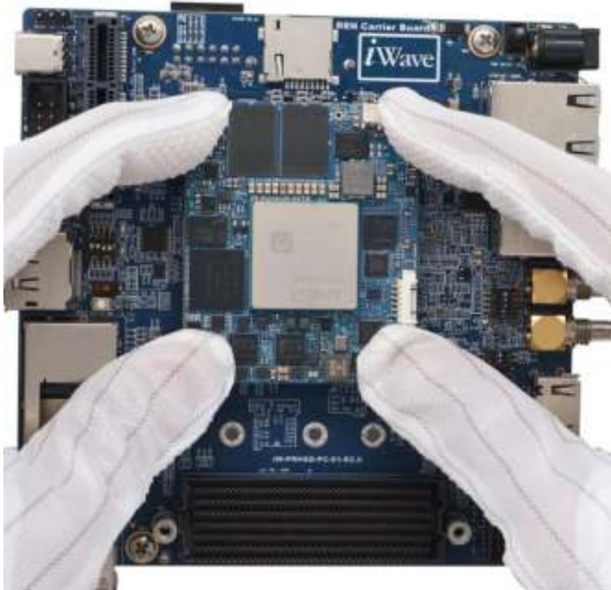
Figure 27: Insertion of SOM in to Carrier Board
