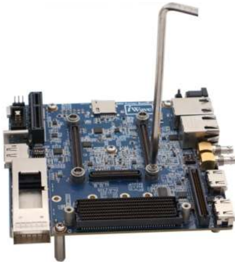
Figure 26: Tightening the of Jack Screw
