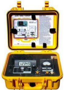
APM Hexseal began its history working with the military. One project example was providing pushbutton switch covers, toggle switch covers, and rotary trim potentiometer covers (zero pot) for an Ordinance/Igniter Tester that's exposed to high moisture conditions (i.e. rain, ocean salt water spray) and therefore must be protected against the elements. A proven method for making these components highly water resistant was essential.
